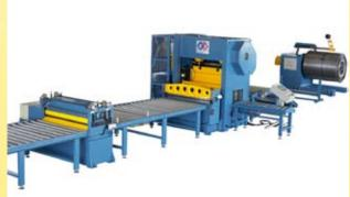
processing thickness ranges from 3.2mm to 8mm and width from 600mm to 1600mm, and a flattener which can be fed sheet with a thickness of 0.3mm-3.2mm.
